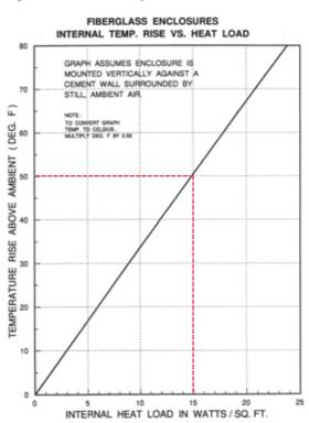
Figure 1. Internal Temperature Rise vs. Heat Load
