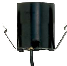
80-1645 Snap-In Socket for 3 1/4"-4" Holders 12" AWM B/W Leads 125°C 660W-250V
