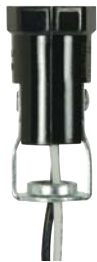
80-1300 26" Leads 80-1398 36" Leads 80-1844 48" Leads 1 1/4" Flange #18 UL 1430 B/W Leads 105°C 1/8 IP-Inside Extrusion Double Leg 75W-125V
