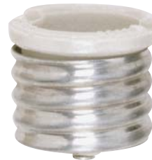
92-406 Mogul to Medium E39 - E26 Reducer 660W-250V
