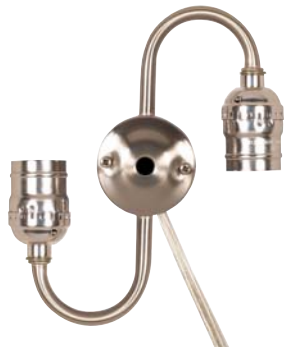
80-1271 Satin Nickel Twin Keyless with 14" 18/2 SPT-2 105°C Clear Silver Wire Internal Wire-18 AWM 105°C 7" Centers 1/8 IP Top and 1/8 IP Bottom 660W-250V
