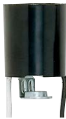
90-1151 10" 80-2095 24" 80-2096 36" AWM B/W Leads 105°C 1/8 IP Hickey 660W-250V
