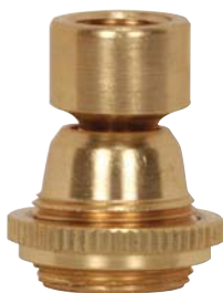
90-2593 Large Hang Straight Swivel 1/4 F x 1/8 M Ring Nut to Seat 1 1/8" 1 1/2" Height Unfinished
