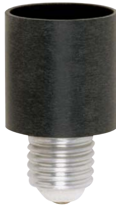
92-414 Medium to Mogul E26 - E39 Extender Overall Ext. 1 3/4" 660W-250V
