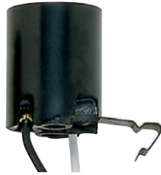
90-595 Snap-In Socket Bracket Extends 3/4" from End of Socket 7" AWM B/W Leads 105°C 660W-250V
