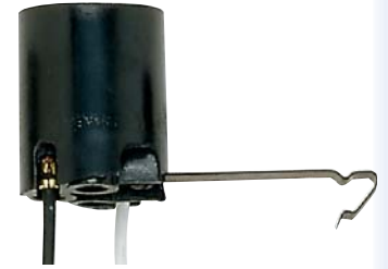
90-542 Snap-In Socket for 8" & 10" Pans Bracket Extends 1 3/4" from End of Socket 8" AWM B/W Leads 105°C 660W-250V
