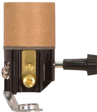
80-2034 2½" 2 Circuit 3 Terminal Turn Knob 1/8 IP Inside Extrusion with Paper Liner 250W-250V
