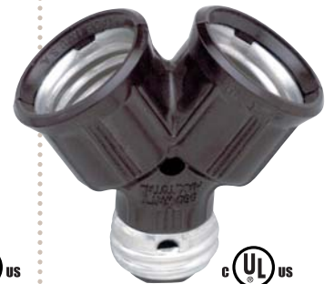
90-1121 Brown 90-2465 Ivory Single to Twin Lampholder 660W Max. Total-250V
