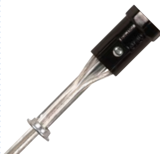
80-1148 3" Flange 24" 18/2 SPT-2 105°C Clear Silver Leads 1/8 IP-Inside Extrusion Single Leg 75W-125V
