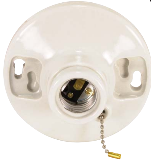
90-443 2 Terminal 90-2638 7" AWM B/W Leads 105°C Glazed Porcelain On-Off Pull Chain Ceiling Receptacle Screw Terminals 250W-250V
