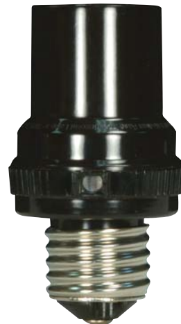
90-2604 Brown Medium to Medium Adapter E26 - E26 with Photocell Overall Ext. 2" 150W-120V (incandescent) 60W-120V (fluorescent) Suitable for Dry or Damp Location
