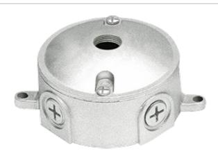
Die cast aluminum wiring box with weatherproof gasket, ground screw, and two sturdy lugs for wall or ceiling mounting.
