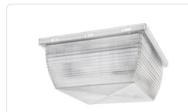
Large size ceiling mount fixture: 26 - 52 Watt compact fluorescent. Reflector is die formed heavy gauge steel in white finish with clear polycarbonate refractor. Lamp supplied.
