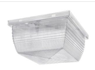
Medium size fixture: 26 and 32 Watt compact fluorescent lamp. Reflector is dieformed heavy gauge steel in white finish with clear vandalproof polycarbonate refractor. Lamp supplied.
