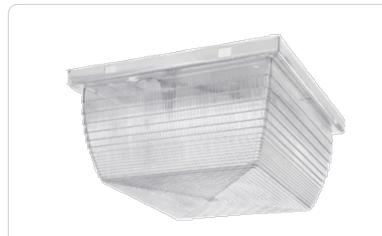
Medium size fixture: 26 and 32 Watt compact fluorescent lamp. Reflector is dieformed heavy gauge steel in white finish with clear vandalproof polycarbonate refractor. Lamp supplied.
