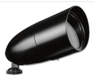
Low voltage MR16 flood with die cast aluminum housing, integral glare shield and tempered lens. Sleek good looks with minimal size. Supplied with 36" SPT-1 cord for installation on low voltage systems. MR16 lamp, 50 Watt max. Lamp not supplied.
