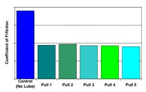
Actual data from the test (above) shows no change in friction coefficient through five water change cycles.
