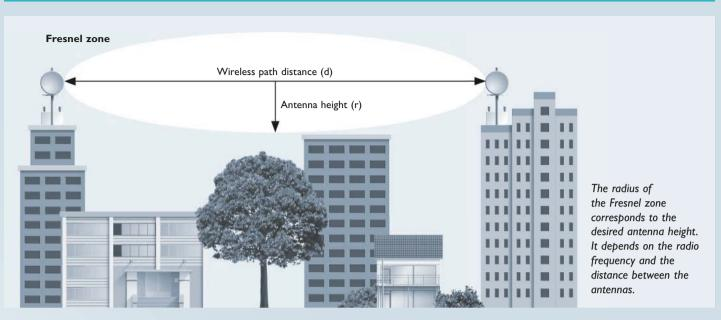
There should be a line of sight, especially in the event of longer distances, between the antennas of the wireless devices.
