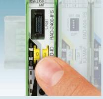
Unique addresses for front modules Set a unique address on the front module by simply turning the thumbwheel.
