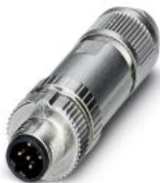
Bus system connector, PROFIBUS (12 Mbps), 2-position, shielded, Plug straight M12 SPEEDCON, Coding: B, Spring-cage connection, knurl material: Zinc die-cast, nickel-plated, external cable diameter 4 mm ... 8 mm
