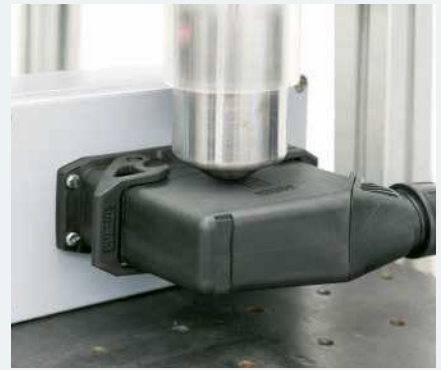
Impact of falling hammer weighing 1.7 kg
