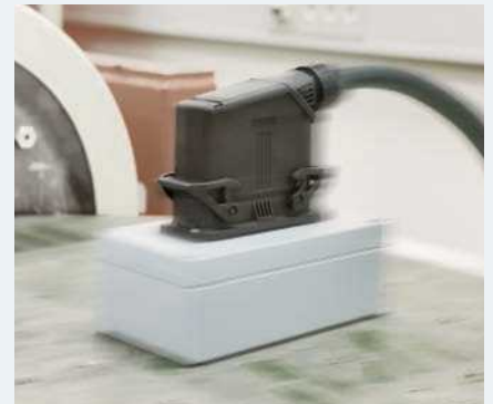
Vibration test according to IEC 60068-2-6
