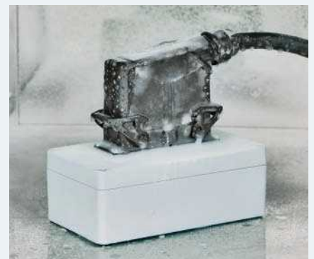
HEAVYCON EVO connector in the climatic chamber at -50°C
