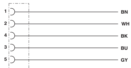
Contact assignment of the M12 sockets
