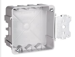
4" Square Box with Threaded Mounting Holes for Wood and Steel Stud Mounting. Three Auto/Clamps each end, 2 on side opposite bracket. Two #8 mounting screws factory installed.
