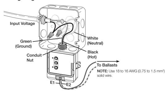
In some applications, a PowPak<sub>TM</sub> module can be installed inside a 4 in x 4 in (102 mm x 102 mm) junction box. For information about how to perform this installation, please see Application Note #423 (p/n 048423).
