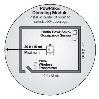
All Wireless Transmitters must be installed within 30 ft (10 m) of the PowPak™ Dimming Module.
