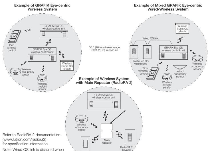
Note: Wired QS link is disabled when the GRAFIK Eye QS control unit is added to a RadioRA 2 system.
