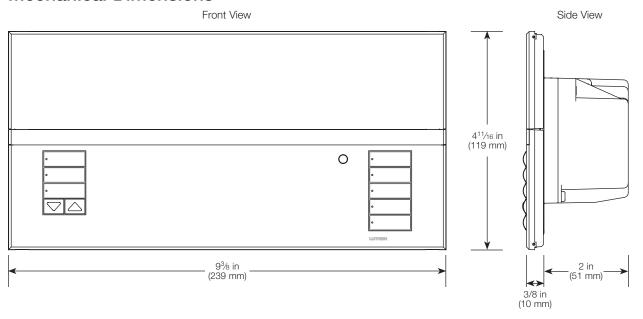
Fits into a 4-gang U.S. backbox, 3½ in (90.4 mm) deep (Lutron P/N 245254) or 3 in (76.2 mm) deep (Lutron P/N 241400)
