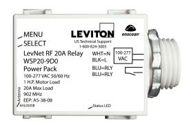
The LevNet RF™ 902 MHz Line Voltage Receiver receives signals from LevNet RF self-powered sensors, switches, and other transmitters to control lighting, and other devices or loads. Self-powered RF technologies eliminate control switch-legwiring, making them an ideal solution for retrofits and new construction. Installation is quick and easy and the receiver mounts with no additional wiring required.
