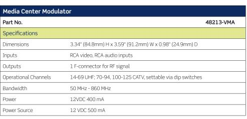
Note: Modulator broadcasts mono audio only. Cannot be combined with digital cable.
