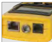
RJ45, F-Connector and RJ11/12 Port
