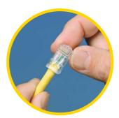
**STEP 7**Slide assembly into plug body.
