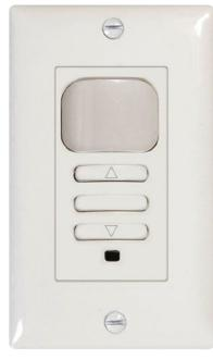
The *LightHAWK*2 Dimming Wall Switch Sensor combines passive infrared (PIR) technology with the additional energy savings of 0-10V dimming. The user can set the occupied level to a predetermined level or set the sensor to activate to the last-used dimming level. With ON/OFF and Dimming Control, the user can easily adjust the light level for their area. This sensor has a coverage area of up to 1,000 square feet and 180° of detection.
