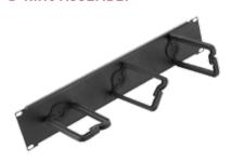
Mounts horizontally on 19-in. racks. Allows grouping vertical cable runs. D-Rings rotate on bracket for easy cable positioning; snap open for easy access for cable updates, yet latch securely. Back plate made of steel with RAL 9005 black polyester powder paint finish; D-Rings are black plastic. Mounting hardware included.
