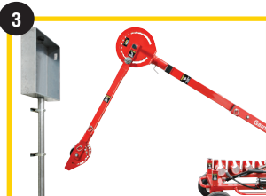
3 Align with conduit, properly adjust booms
