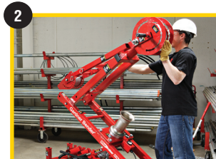
2 Flip booms into position and lock
