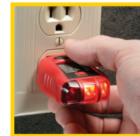
Tests outlets protected by GFCIs
