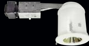
5" Remodel Housing EL5RLV • Height: 7 1/2" • Opening: 5 1/2" • Lamp: 12V 75W MR16 • UL damp location listed • UL feed through listed
