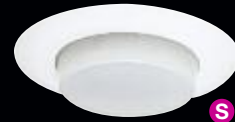
Shower Trim with Acrylic Drop Lens and White Socket Reflector EL319W White Plastic Ring Lamp: 60W A19 O.D.: 8" S NEW!
