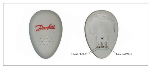
Simplify your installation process using the Little Buzzer by Danfoss! The Little Buzzer is designed to monitor Danfoss heating mats and/or cables during the installation process and sounds an alarm if the heating elemnts are cut or damaged. This allows easy repair before the floor coverings are laid. The device is battery powered (batteries included).
