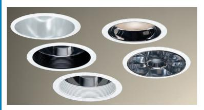
**Reflectors** PDS offers a full range of reflector options including open, open wall wash, baffle and lens with a choice of patterns. One-piece construction avoids internal losses and light leaks that occur at the ceiling line. PDS provides a 5/8" overlapped flange to cover the ceiling cutout and provide a gap free aperture with no light leaks around the flange or visible cut edge of ceiling tile.
