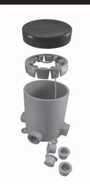
A cylindrical enclosure designed to be embedded in a concrete floor with some excess length remaining above the plane of the floor. Excess is trimmed flush with the concrete. Sold as a kit with one leveling ring, 4 blank hubs (Stoppers), 4 reducing bushings and one polyethylene temporary pour lid
