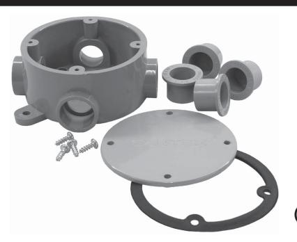
A 4" round enclosure with four entrance hubs which is surface mounted to a wall or ceiling to terminate a conduit run or join two to four conduits at a common point and to allow space for wire splices. Four screws secure a blank cover to the box.
