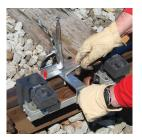
• Used to remove the slag from the crucible area of the mold after making a ERICO CADWELD connection
