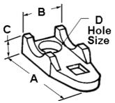
Dimension A in Inches: 5-3/4 Dimension B in Inches: 2-7/16 Dimension C in Inches: 3/4 Dimension D in Inches: 3/4
