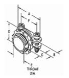
Dimension A in Inches: 1-5/16 Dimension B in Inches: 7/16 Dimension C in Inches: 3/8 Dimension D in Inches: 15/16 Dimension E in Inches: 5/8 Dimension F in Inches: 15/16
