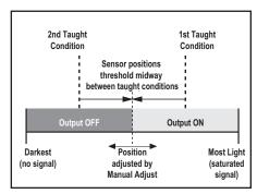
Figure 2. Static TEACH (Light Operate shown)
