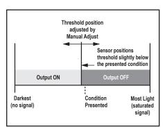
Figure 7. Single-Point Light SET (Dark Operate shown)
