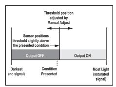
Figure 9. Single-Point Dark SET (Light Operate shown)
