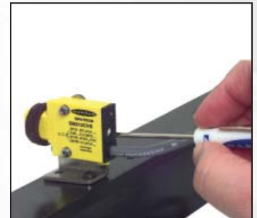
Figure 54. Teachable sensors with microprocessors are useful when contrast is low
