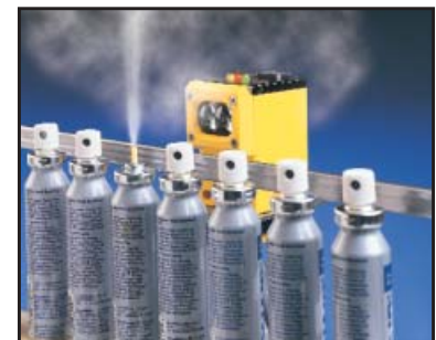
Figure 17. Fiber optic use in a hostile environment
