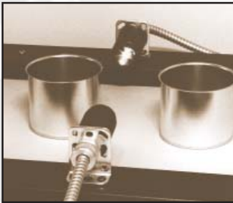
Figure 1. Early photoelectric sensors used an incandescent light bulb; advanced technology has resulted in ever-smaller LED-based sensors
