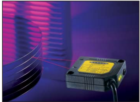
Figure 31. The narrow, sharply defined sensing beam of a PicoDot laser diode sensor detects the edge of a semiconductor wafer in a wafer cassette mapping application
