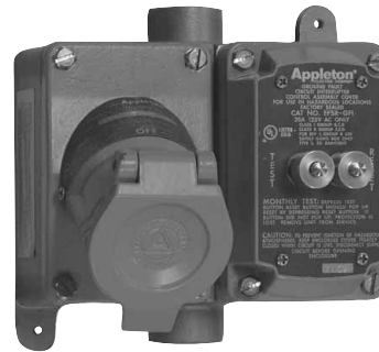
EFSR–GFI cover installed on two–gang EFD box together with U–Line 20 Amp, 125 Vac factory sealed receptacle. Receptacle listed for Class I, Groups C and D, Class II, Groups F and G, and Class III.
