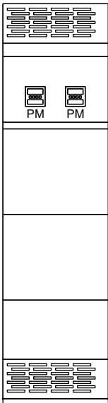
Power Meter for I-Line Circuit Breakers in 24 in. (610 mm) Wide Auxiliary Section
