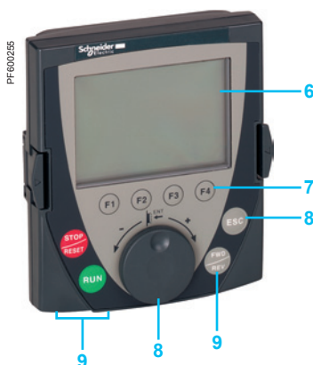
Remote graphic display terminal
