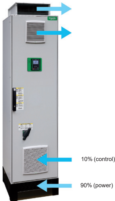
Cooling system with two separate air flows
