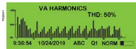
PowerLogic ION8650 front panel harmonic display.
