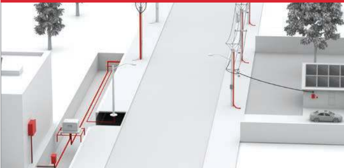
Overhead and Underground Power Distribution
